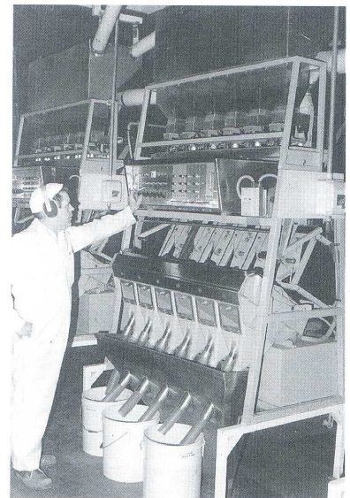
Jim Holden adjusting the Sortex Bean Sorting Unit - Culinary Plant 1980's.
